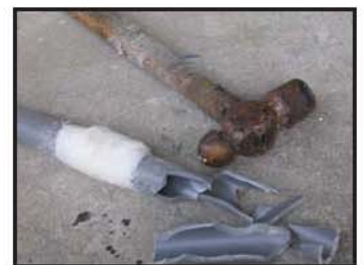
• Repaired area does not fail under impact test
